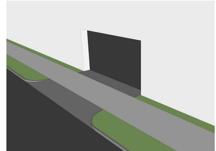
**Figure 4** Continuing the sidewalk surface across the curb cut can lessen the impact of the cuts.
